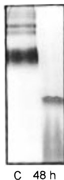
Figure 1. Native PAGE of the control (C) and legumin plus linoleic acid (48 h) after incubation at pH 9.0 and 37 °C for 48 h.
